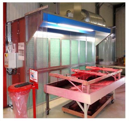
VALINOX NUCLEAIRE wished install an extraction booth in order to **protect its operators** during liquid penetrant inspection.
