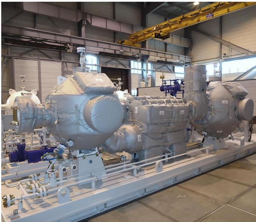
Clyde was looking for a means of insulating pump bodies both **thermally and acoustically**, while still guaranteeing quick access to the machines.
