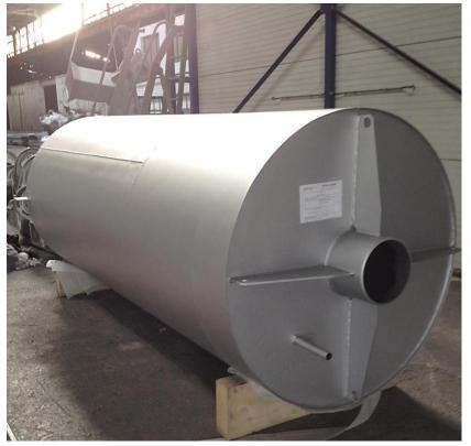
BERTSH, a world renowned Austrian company, entrusted dB Vib Engineering with the **design and manufacture of two atmospheric discharge silencers**.
