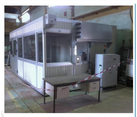
The chemical extraction of minerals is associated to **complex and sensitive equipments** in the whole process. AREVA MINES wanted to purchase a safe and well-instrumented **test bench** in order to **validate the vibratory behaviour of its machines** after maintenance, before to reinstall them in production.
